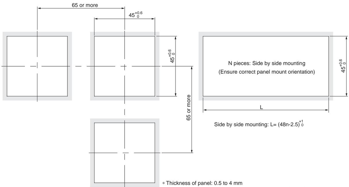
\* Thickness of panel: 0.5 to 4 mm
