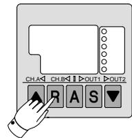
Press the button "R" for at least 2 seconds but no longer than 3 seconds. This clears the auto shift function.
