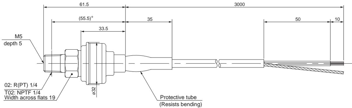
\* Reference dimensions after thread installation
