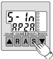
When the initial condition for adsorption confirmation are met, press the button "S". Press the ▼ button when it is not required to calibrate OUT2.
