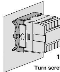
Turn screw 1/4 to 1/2 turn after panel makes contact with the sealing surface of the PSE.
