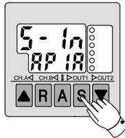
When the initial conditions for adsorption confirmation are met, press the button "S". Press the ▼ button when it is not required to calibrate OUT1.
