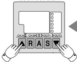
Press the ▼ and ▲ buttons simultaneously for at least 3 seconds. Display starts to blink.
