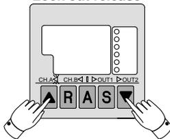
Press the ▲ and ▼ buttons simultaneously for at least 3 seconds. Lock out is released. During malfunction lockout is released automatically.
