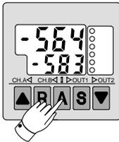
Press the button "A" for 3 to 6 seconds for selected channel, and for more than 6 seconds for not selected channel.
