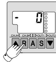
Press the button "R" for at least 3 seconds to reset the display to zero. If pressure is higher than ±2% of rated pressure, reset of the display is not possible.
